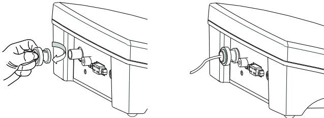
REF socket is for separate reference electrode. (e.g. STREF1)
