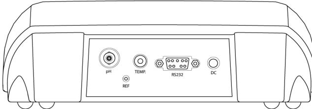
For ST310 electrode connect to the BNC and Cinch socket. For 2-in-1 pH electrode (e.g. ST210) you only need to connect the BNC.
