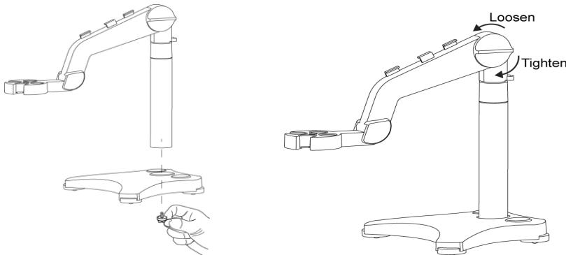
After adjusting the tension knob to some extent, you can move the upper arm up and down. When the pH electrode is installed on the arm, the storage bottle of pH electrode fits into the base hole.
